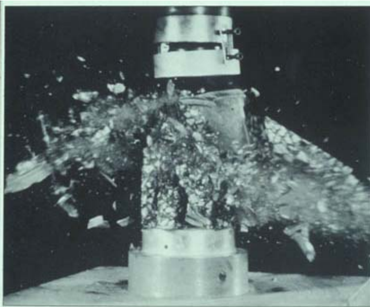
A cylinder of high-strength concrete is tested to failure.
